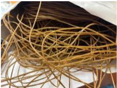
PLA/PBSA 80/20 + 10 wt.% Tangerine residue POST-extraction
