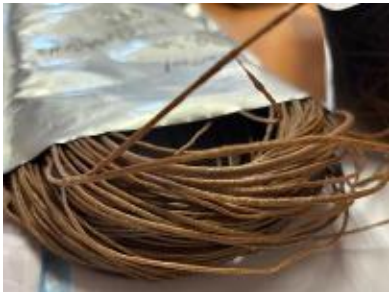
PLA/PBSA 80/20 + 10 wt.% Tangerine residue PRE-extraction
