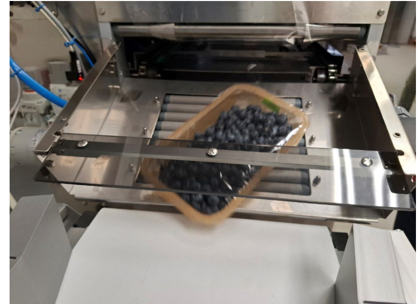
Figure 5. Packaging of blueberries into developed PLA-apple fiber tray (Slice-Pack-Line, Bizerba) (own illustration, SPI)
