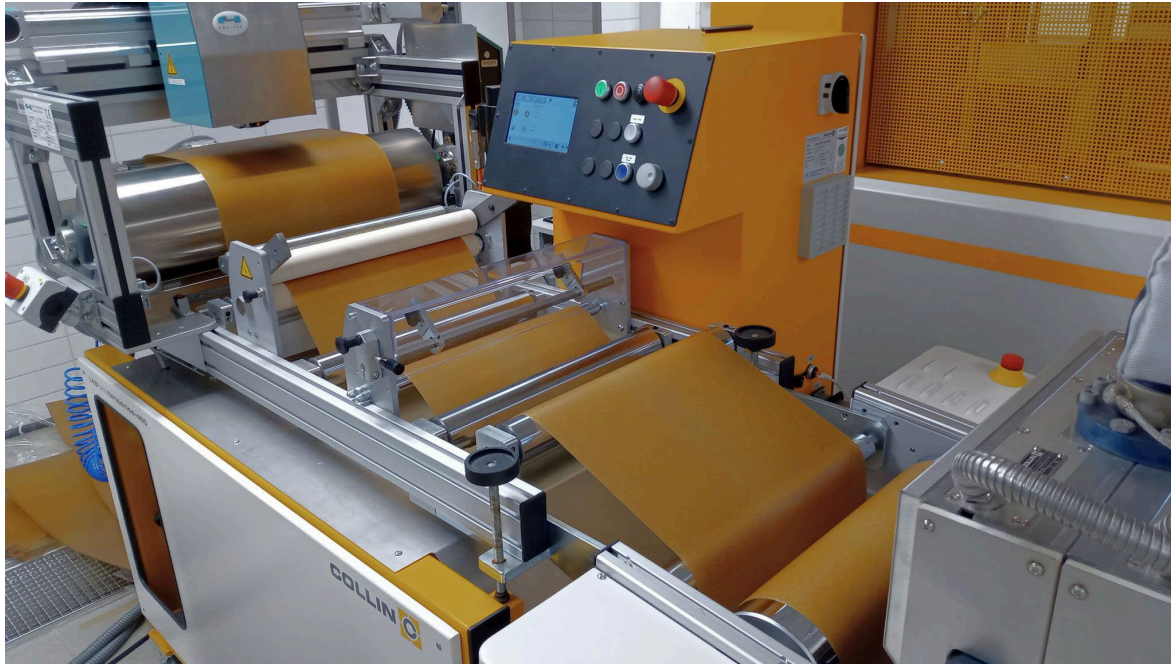
Figure 4. Compounder with flat film system – production of PLA-wood fiber films (left image) or PLA-apple fiber film (right image) (Sustainable packaging institute, own source)
